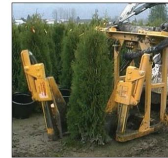
Horse-shoe Platform to hold the soil in place while retracting the blades
