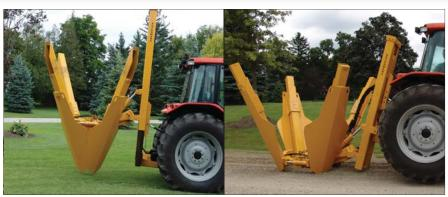
Dutchman Lift-Mast Assembly for mounting a Tree Spade to rear of any tractor.
